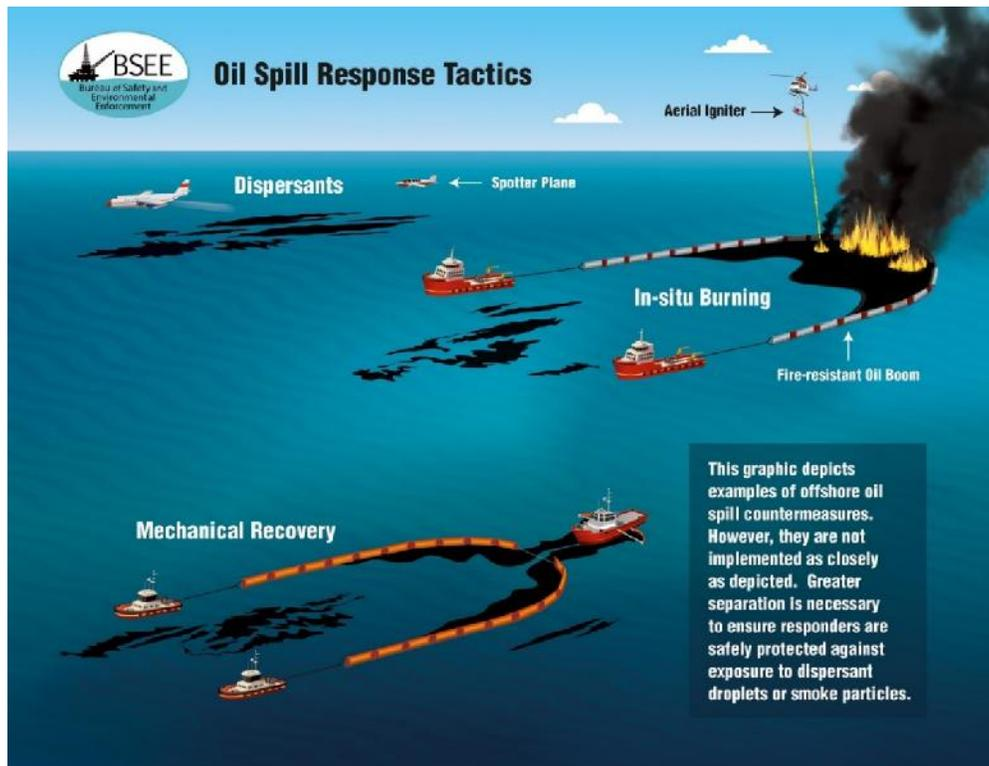
Figure 2.21. Examples of offshore oil spill response options (Source: BSEE 2023).
