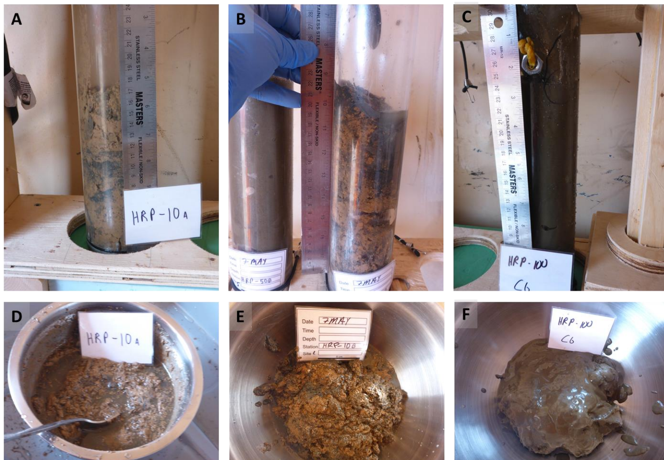
Figure 3-5 Grid box push core and associated extruded samples for A) station HRP-10A (drill cuttings), B) station HRP-10B (drill cuttings), C) station HRP-100, D) station HRP-10A (drill cuttings), E) station HRP-10B (drill cuttings), and F) station HRP-100.
