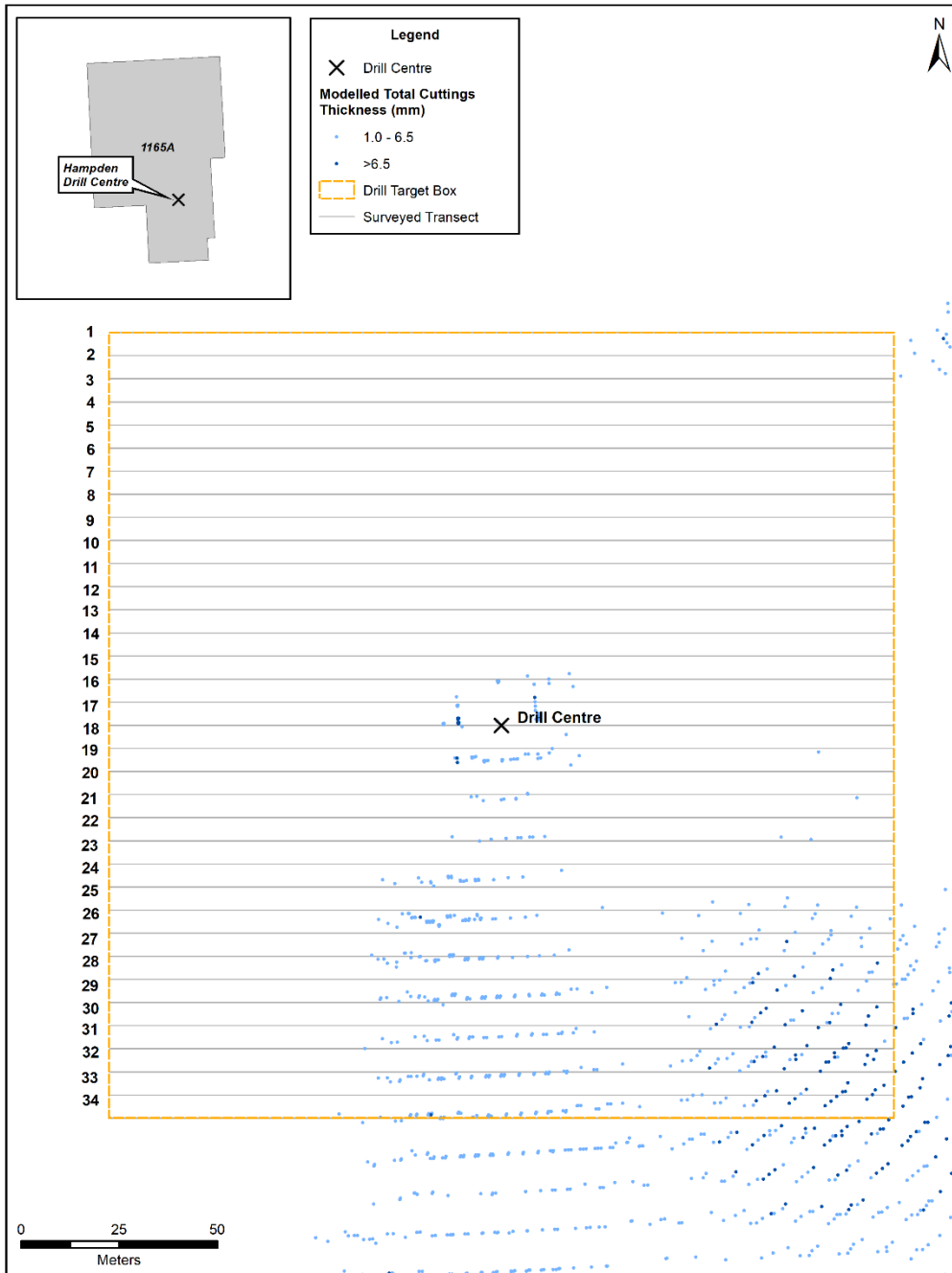
Figure 2-2 Post-drilling survey design at EL1165A.
