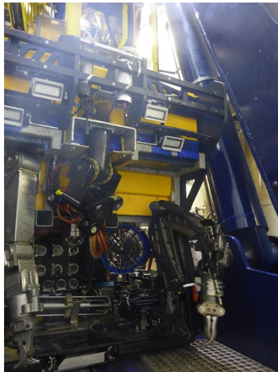
Figure 2-1 Millennium 191 ROV used for the 2020 EL 1165A post-drilling survey
